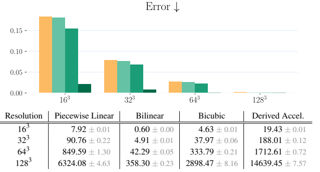
Figure 3: Top: Comparison of cross product residuals (lower is better) for: piecewise linear (●), bilinear clipping (●), bicubic clipping (●), and bicubic clipping with derived acceleration (●). Bottom: Comparison of the total runtime (serial) in milliseconds.
