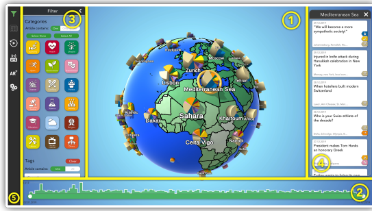
Figure 1: Main Window Sections: (1) globe visualization, (2) timeline with histogram, (3) filtering panel, (4) article details, (5) menu.
